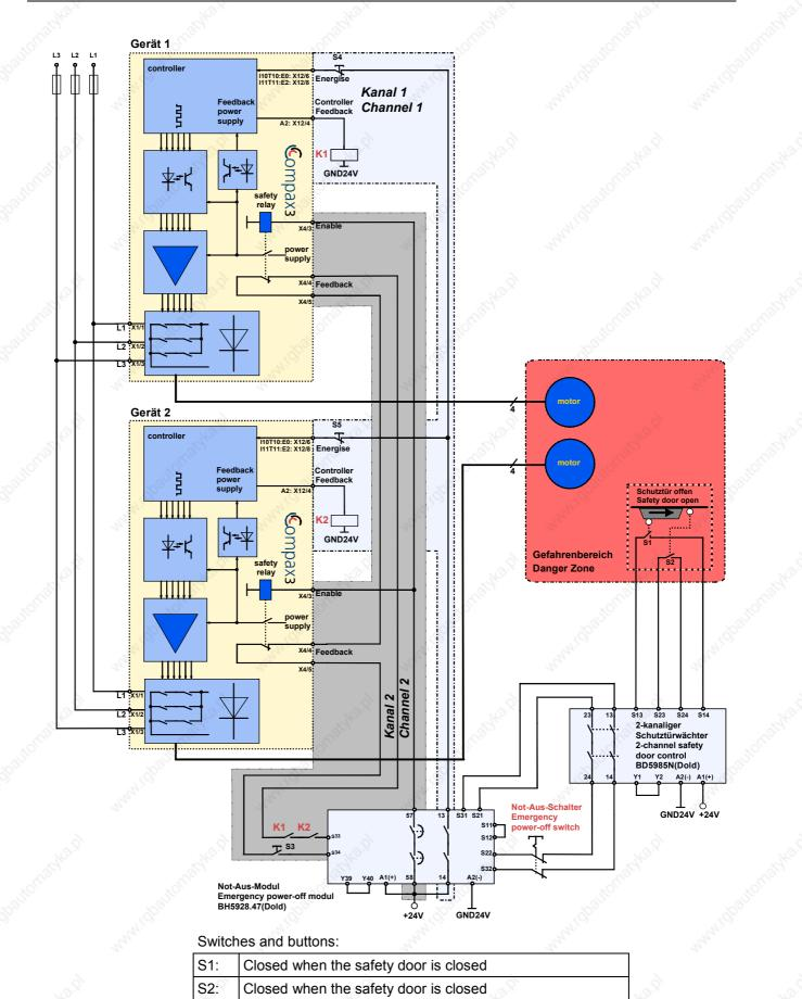
Guide Device 1 to a currentless state (error acknowledge)
