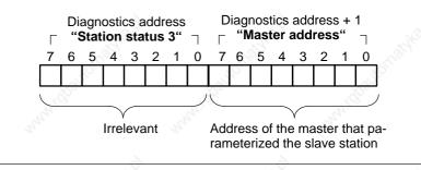
Figure 6-5 Structure of the "Station Status 3 and Master Address" Diagnostics Word
