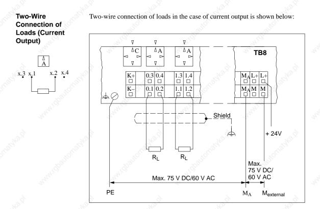
Figure 9-24 2-Wire Connection of Loads in the Case of Current Output
