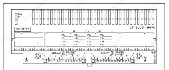
Figure 8-42 Front Elevation: ET 200B-16RO-AC (6ES7 132-0HH00-0XB0)
