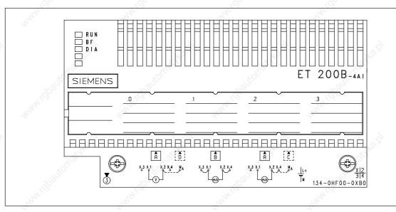
Figure 9-15 Front Elevation: ET 200B-4AI (6ES7 134-0HF00-0XB0)
