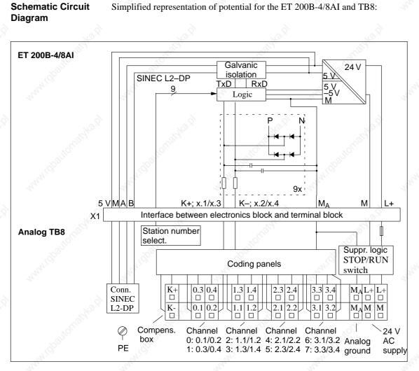
Figure 9-14 Schematic Circuit Diagram: ET 200B-4/8AI (6ES7 134-0KH00-0XB0) and TB8
