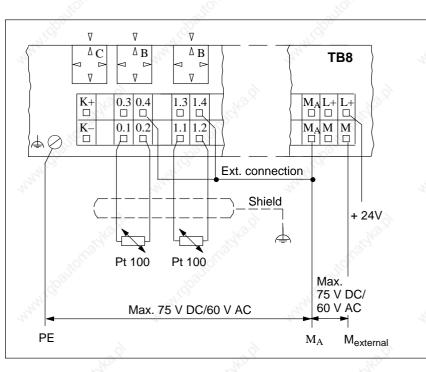
Figure 9-9 Connection of Resistance Thermometers (Pt 100) with 2-Wire Connections (Ground-Referenced Measurement)
