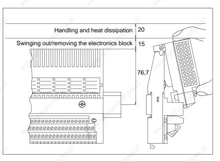
Figure 3-1 Clearances Required for Installation of the Electronics Block
