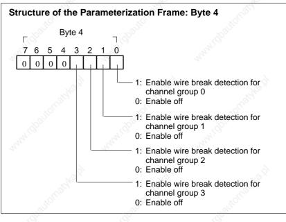
Figure 4-5 Structure of the Parameterization Frame of the ET 200B-4/8AI: Byte 4
