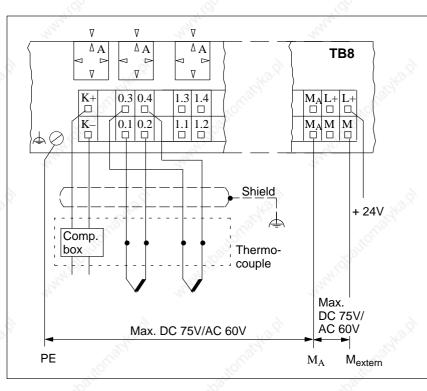
Figure 9-6 Connection of Thermocouples with a Compensating Box (Floating-Ground Measurement)
