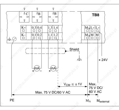
Figure 9-18 Two-Wire Connection of Current Sensors (Floating-Ground Measurement)
