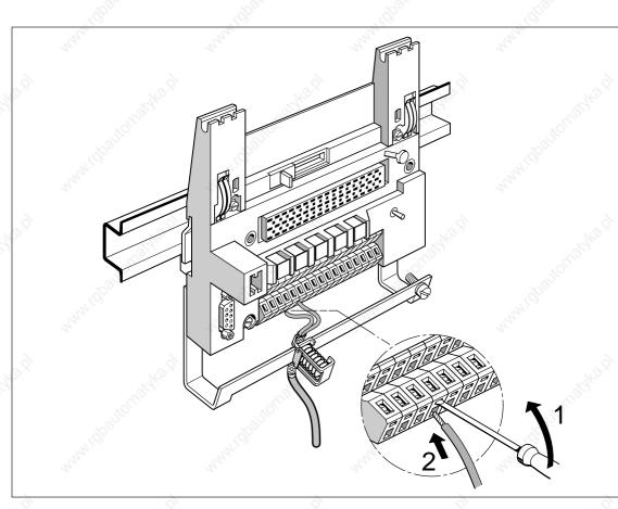
Figure 3-12 Securing the Wire in a Spring-Loaded Connection
