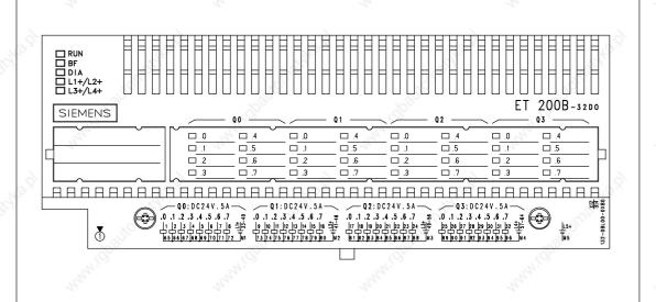
Figure 8-26 Front Elevation: ET 200B-32DO (6ES7 132-0BL00-0XB0)
