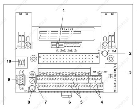
Figure 2-1 TB1/DC Terminal Block
