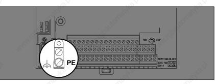
Figure 3-7 Both Screws Tightened in a Grounded Configuration
