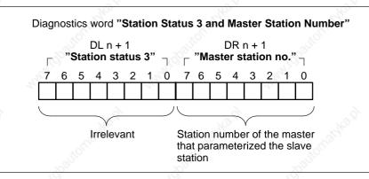
Figure 6-14 Structure of the "Station Status 3 and Master Station Number" Diagnostics Word
