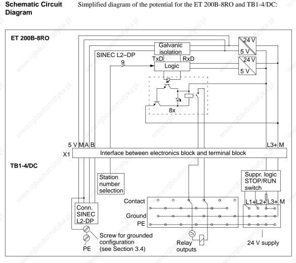
Figure 8-31 Schematic Circuit Diagram: ET 200B-8RO (6ES7 132-0GF00-0XB0) and TB1-4/DC
