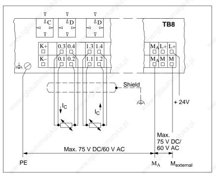
Figure 9-11 Connection of Resistance Thermometers (Pt 100) with 4-Wire Connections (Ground-Referenced Measurement)
