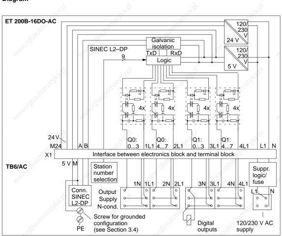
**Schematic Circuit** Simplified diagram of the potential for the ET 200B-16DO-AC and TB6/AC: **Diagram**
