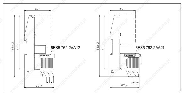
Figure 8-13 Dimension Drawing: Side Elevation of Terminal Block TB6/AC with SINEC L2 Bus Connector (6ES5 762-2AA12 and 6ES5 762-2AA21)
