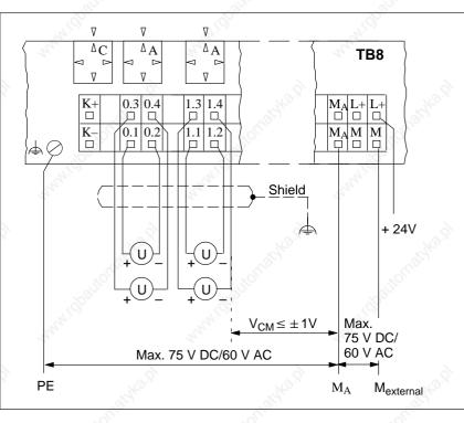
Figure 9-12 Two-Wire Connection of Voltage Sensors to 6ES7 134-0KH00-0XB0 (Floating-Ground Measurement)
