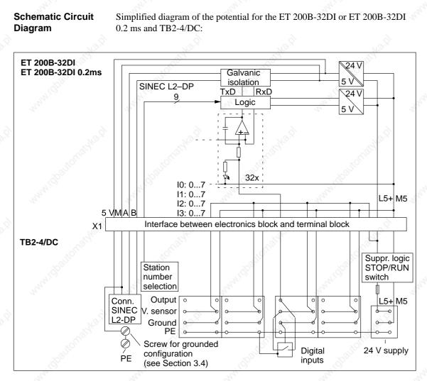
Figure 8-19 Schematic Circuit Diagram: ET 200B-32DI (6ES7 131-0BL00-0XB0) or ET 200B-32DI 0.2 ms (6ES7 131-0BL10-0XB0) and TB2-4/DC
