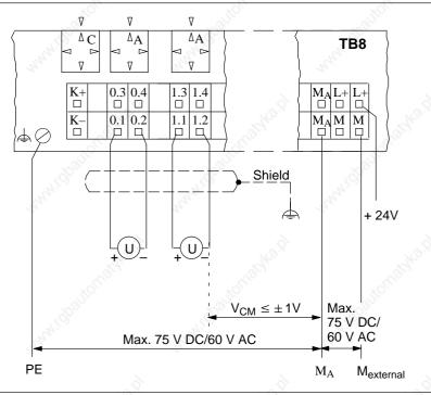
Figure 9-16 Two-Wire Connection of Voltage Sensors to 6ES7 134-0HF00-0XB0 (Floating-Ground Measurement)
