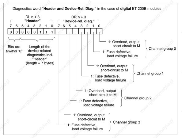
Figure 6-16 Structure of the "Header and Device-Related Diagnostics" Diagnostics Word in the Case of Digital ET 200B Modules"
