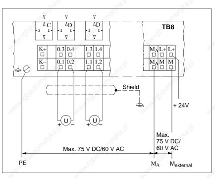
Figure 9-17 Two-Wire Connection of Voltage Sensors 6ES7 134-0HF00-0XB0 (Ground-Referenced Measurement)
