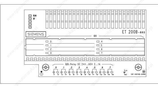
Figure 8-29 Front Elevation: ET 200B-8RO (6ES7 132-0GF00-0XB0)
