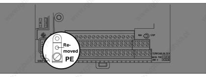
Figure 3-10 Upper Screw Removed in an Ungrounded Configuration
