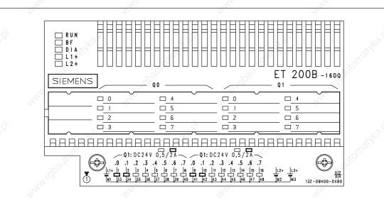
Figure 8-20 Front Elevation: ET 200B-16DO (6ES7 132-0BH00-0XB0)
