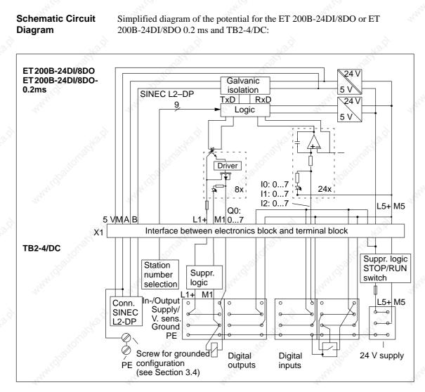
Figure 8-37 Schematic Circuit Diagram: ET 200B-24DI/8DO (6ES7 133-0BN00-0XB0) or ET 200B-24DI/8DO 0.2 ms (6ES7 133-0BN10-0XB0) and TB2-4/DC
