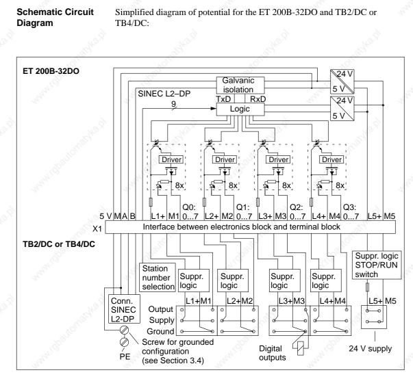
Figure 8-27 Schematic Circuit Diagram: ET 200-B-32DO (6ES7 132-0BL00-0BX0) and TB2/DC or TBA/DC
