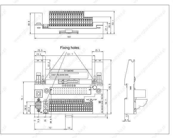
Figure 8-3 Dimension Drawing: Terminal Block TB3/DC (Spring-Loaded Terminal)
