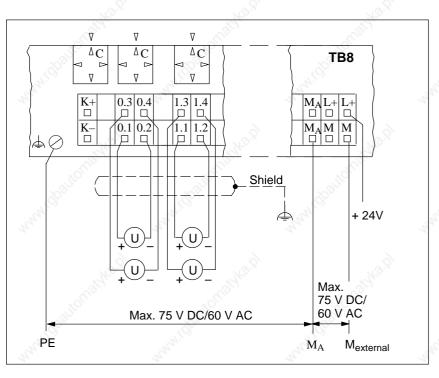
Figure 9-13 Two-Wire Connection of Voltage Sensors to 6ES7 134-0KH00-0XB0 (Ground-Referenced Measurement)
