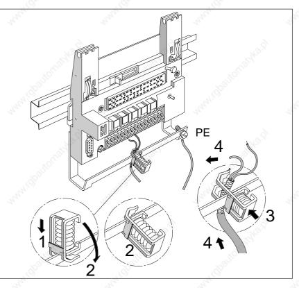
Figure 3-13 Shield Connecting Element on Terminal Block TB8
