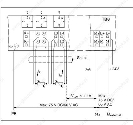
Figure 9-10 Connection of Resistance Thermometers (Pt 100) with 4-Wire Connections (Floating-Ground Measurement)
