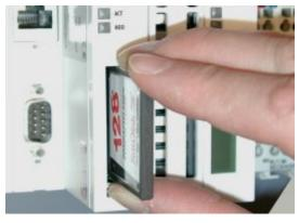
FIG2: Removing the CF card
