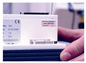
FIG1: Ejecting the CF card
