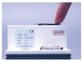
FIG3: Inserting the CF card
