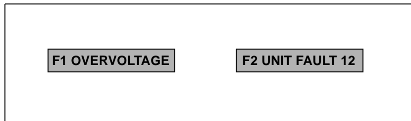
Figure 8-1 Examples of fault indications in the fault memory.
