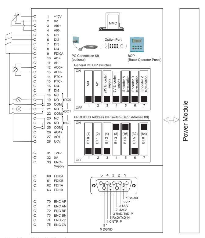
Figure 3-4 CU240S DP-F block diagram
