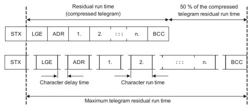
Figure 6-21 Residual Run Time and Character Delay Time
