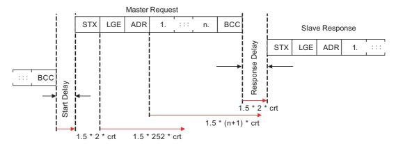
Figure 6-23 Timeout Checks on USS Slave
