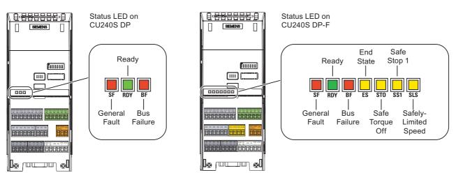
Figure 7-1 State LED on the CU240S, CU240S DP, CU240S DP-F, CU240S PN
