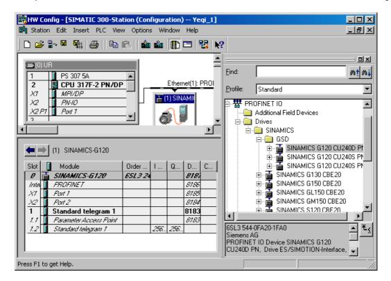
3. Double click onto "SINAMICS G120" to add the G120 as I/O device to the subnet. The SINAMICS G120 is added in the station window.
