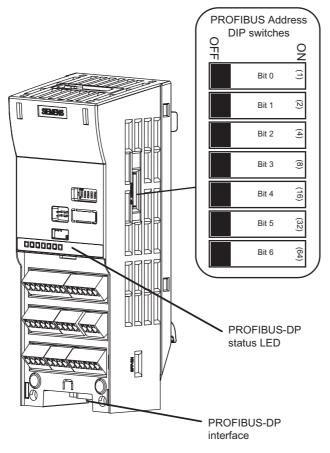
Figure 6-7 PROFIBUS DP address DIP-switches
