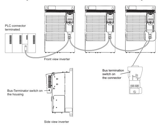
Figure 4-4 PROFIBUS network with bus termination
