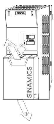
Figure 4-2 Removing the Control Unit terminal cover
