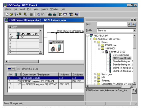
Figure 6-9 G120 inverter with fail-safe functions and a standard protocol in HW config of SIMATIC S7
