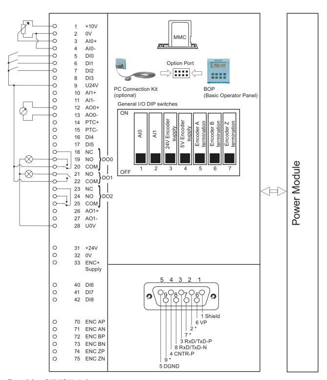
Figure 3-2 CU240S block diagram
