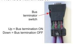
Figure 4-5 PROFIBUS DP bus termination switch
