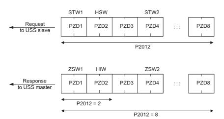
Figure 6-24 Process data channel
