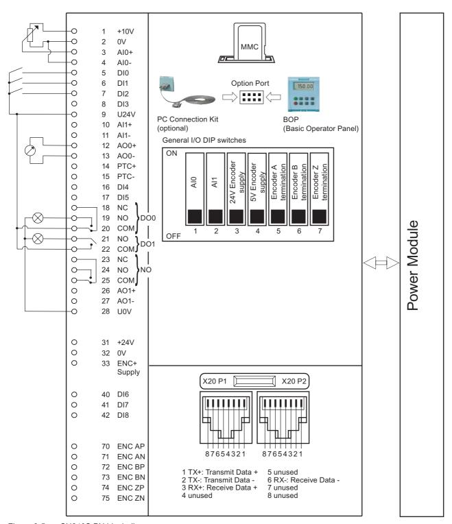
Figure 3-5 CU240S PN block diagram
