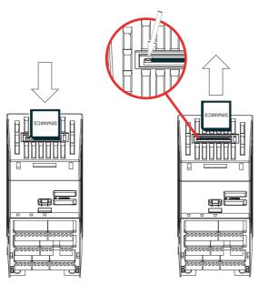
Figure 5-5 Fitting and Removing the MMC
