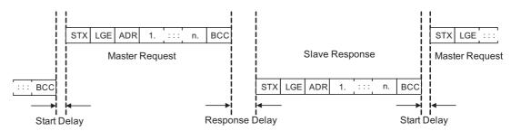
Figure 6-22 Start Delay and Response Delay
