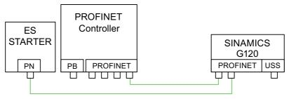
Figure 4-8 Topology 2: direct connection
