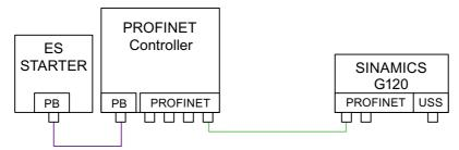
Figure 4-9 Topology 3: Routing
