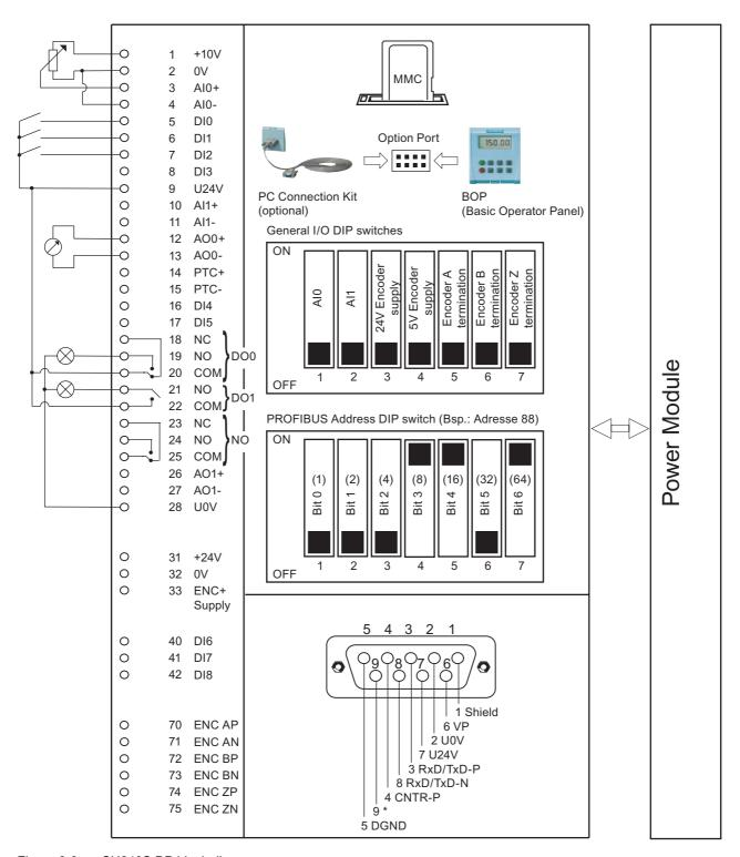
Figure 3-3 CU240S DP block diagram
