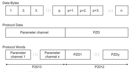
Figure 6-19 USS Application Data
