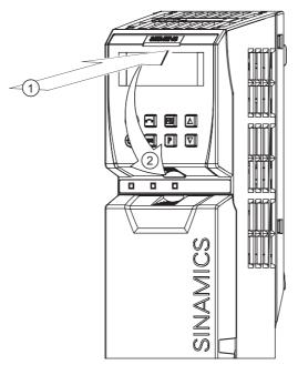
Figure 5-4 Fitting the BOP to the CU
