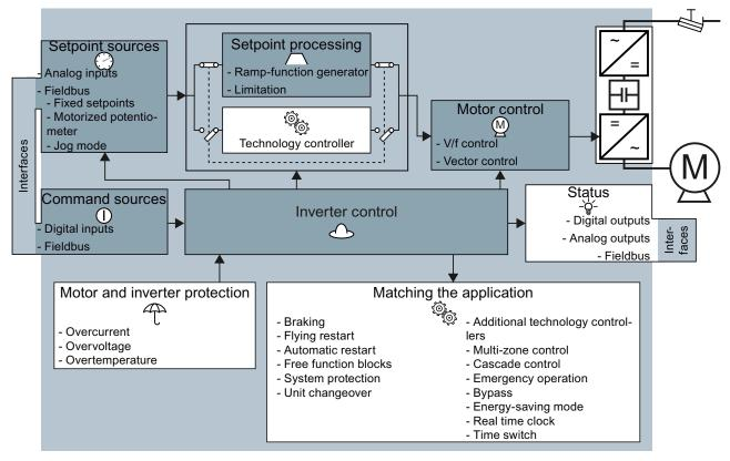
Figure 7-1 Overview of inverter functions
