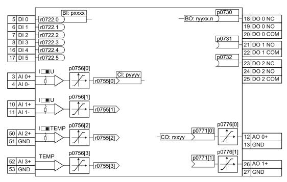
Figure 5-1 Internal interconnection of the inputs and outputs
