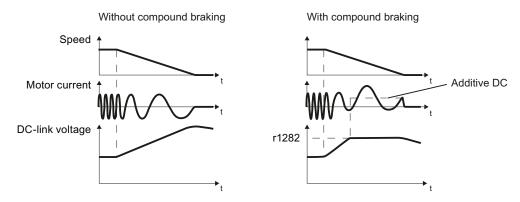
Figure 7-12 Motor brakes with and without active compound braking
