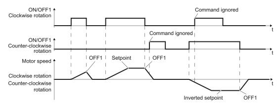
Figure 7-3 Two-wire control, method 2
