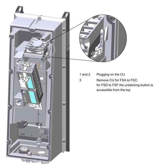
Figure 3-8 Locate the CU on the PM
