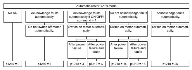
Figure 7-16 Selecting the automatic restart mode
