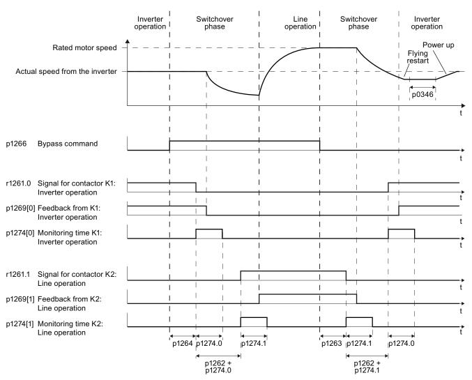
Figure 7-21 Bypass control independent of the speed via a control signal (p1267.0 = 1)
