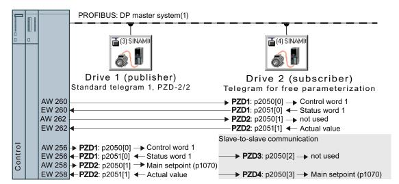
Figure A-5 Communication with the higher-level control and between the drives with slave-to-slave communication
