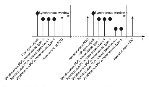
Figure 6-13 Principle of synchronous and asynchronous transmission
