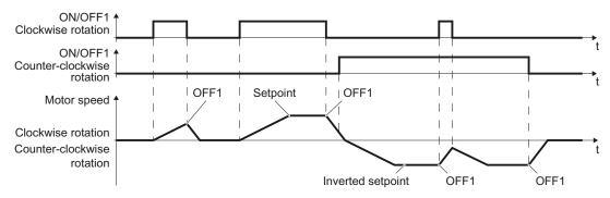
Figure 7-4 Two-wire control, method 3
