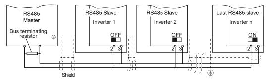
Figure 6-4 Communication network via RS485
