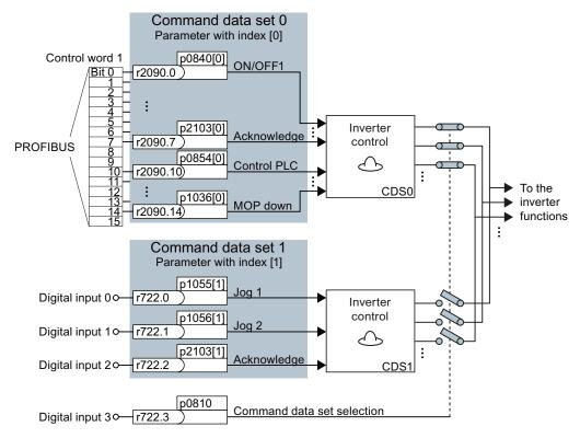
Figure 7-8 Example for the various command data sets
