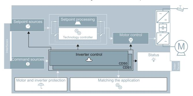
Figure 7-7 CDS switchover in the inverter
