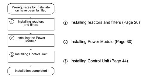
You will find details on the installation in the Internet: Hardware Installation Manual (http://support.automation.siemens.com/WW/view/en/30563173/133300).
