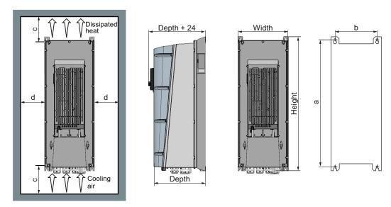
Figure 3-1 Drilling pattern for PM230
