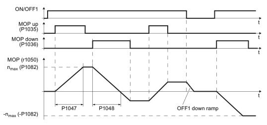
Figure 7-9 Function chart of motorized potentiometer
