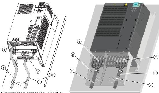
Example for a connection without a shield plate via an external filter
