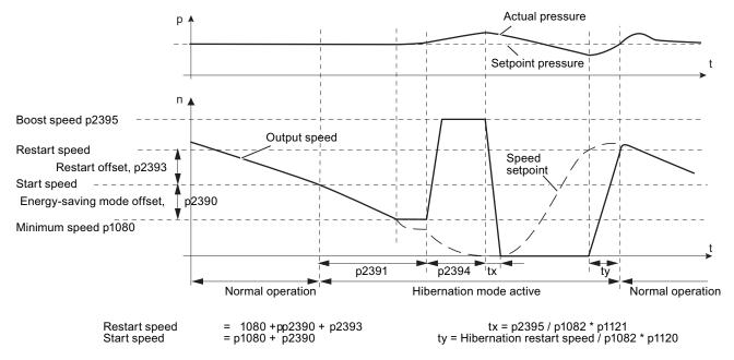
Figure 7-24 Energy-saving mode using an external setpoint with boost
