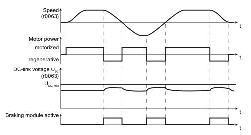
Figure 7-13 Simplified representation of dynamic braking with respect to time
