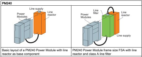
The line-side reactors are equipped with terminals while the reactors on the Power Module side are equipped with a prefabricated cable. In the final installation position, the mains terminals are at the top on frame sizes FSA to FSC, and at the bottom on frame sizes FSD to FSE.
