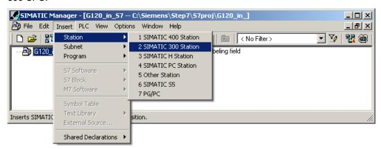
Figure A-1 Inserting a SIMATIC 300 station into a STEP 7 project
