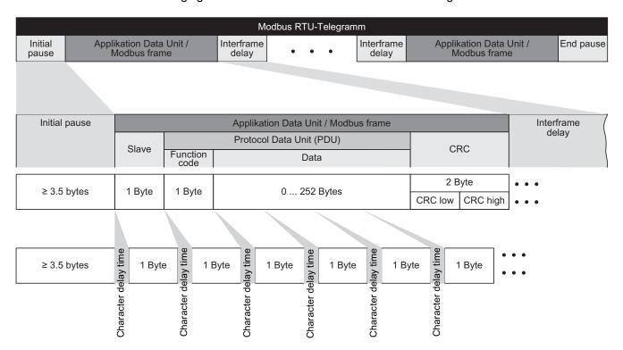
Figure 6-12 Modbus with delay times
