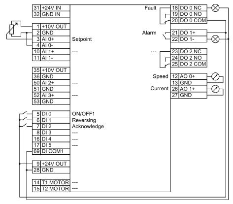
Figure 4-2 Wiring a CU230P-2 HVAC or CU230P-2 CAN to use the factory settings
