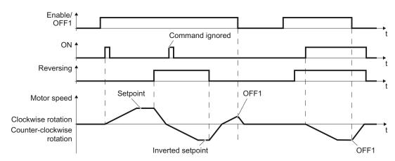
Figure 7-6 Three-wire control, method 2
