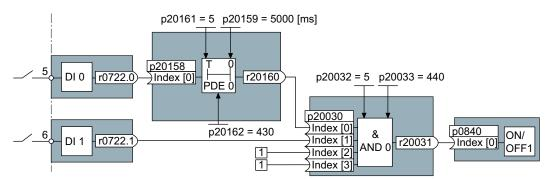
Figure 1-4 Example: Signal interconnection for interlock
