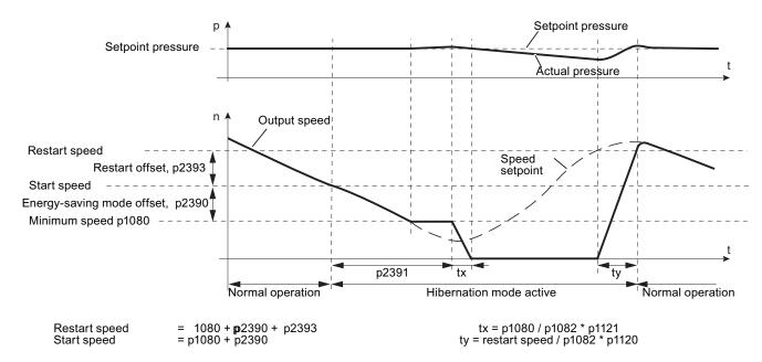
Figure 7-25 Energy-saving mode using an external setpoint without boost
