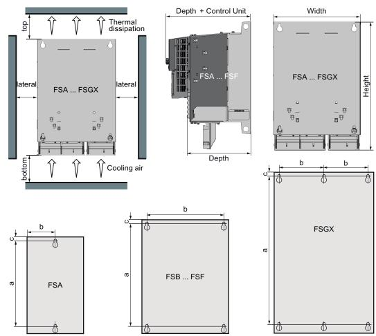
Figure 3-2 PM240 drilling pattern
