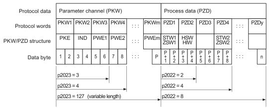
Figure 6-6 USS user data structure
