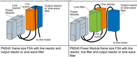
In installations containing more than two base-type system components (e.g. line filter + line reactor + output reactor), the components must be installed to the side of the Power Module whereby the line reactor and line filter are installed under the Power Module and the output reactor to the side.
