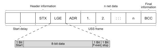
Figure 6-5 Structure of a USS telegram
