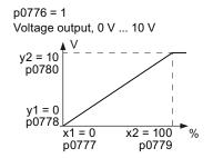
Figure 5-3 Examples for scaling characteristics
