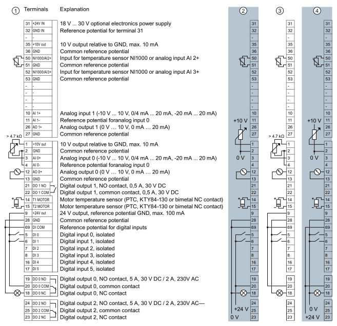
The wiring of the terminal strip is not shown completely, but as example for each terminal type.
