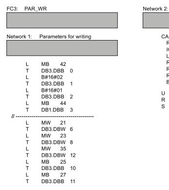
Write request: SFC CALL 58 REQ :=M9.1 IOID :=B#16#54 LADDR :=W#16#170 RECNUM :=B#16#2F RECORD :=P#DB3.DBX0.0 BYTE 14 RET\_VAL :=MW10 **BUSY** :=M8.1 8.1 M R Μ 9.1 S Μ 9.3
