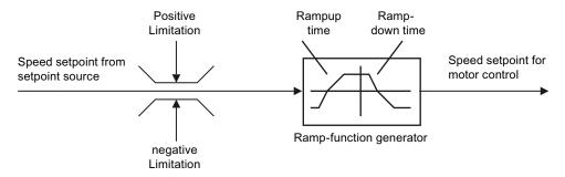
Figure 7-10 Setpoint processing in the inverter
