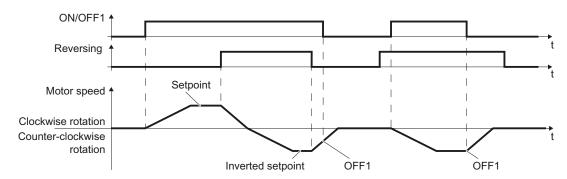
Figure 7-2 Two-wire control, method 1
