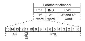
Figure 6-2 PKE - 1st word in parameter channel
