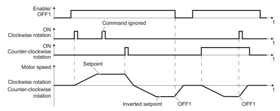
Figure 7-5 Three-wire control, method 1
