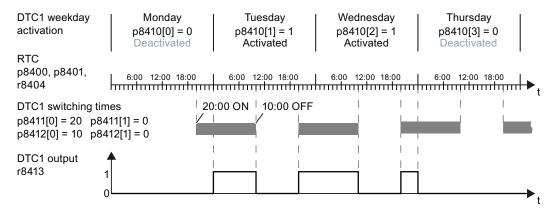
Figure 7-20 Time behavior of the time switch using example DTC1
