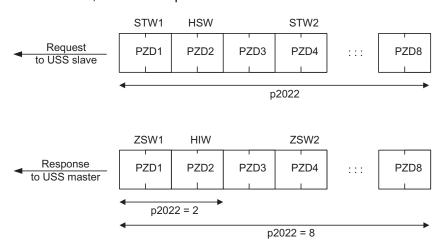
Figure 6-9 Process data channel
