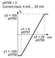
Figure 5-2 Examples for scaling characteristics
