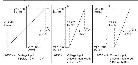
Figure 5-1 Examples for scaling characteristics
