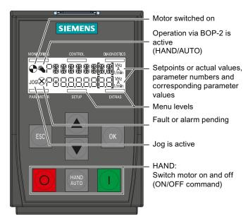
Figure 4-7 Meaning of the display in the BOP-2
