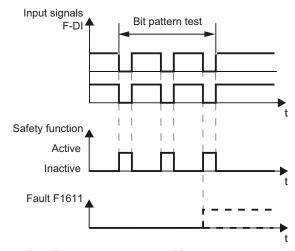
Figure 7-25 Inverter response to a bit pattern test
