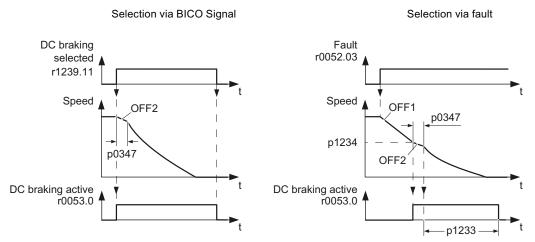
Figure 7-8 Principle of operation of the DC braking
