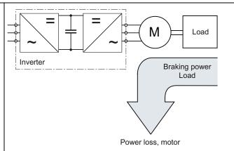
The regenerative energy is converted to heat in the motor.
