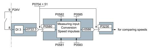
Figure 7-7 Speed deviation monitoring by means of digital input DI3
