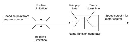
Figure 7-4 Setpoint calculation in the inverter
