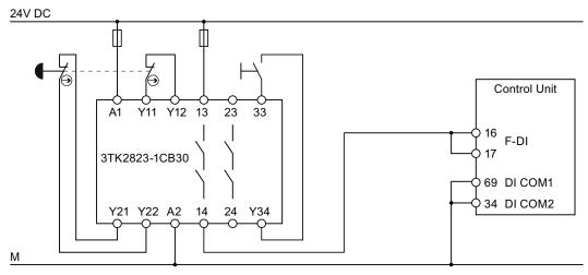
Figure 7-22 Connecting a safety relay, e.g. SIRIUS 3TK28
