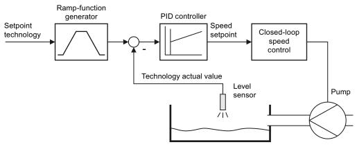
Figure 7-18 Example: technology controller as a level controller
