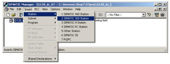
Figure 6-1 Inserting a SIMATIC 300 station into a STEP 7 project
