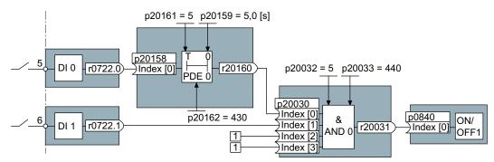
Figure 1-4 Example: Signal interconnection for interlock
