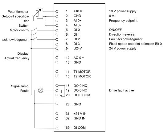
Figure 4-3 CU240B-2: Wiring example for the factory settings
