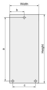
Figure 3-2 Dimensions and drilling pattern, PM240-2 IP20
