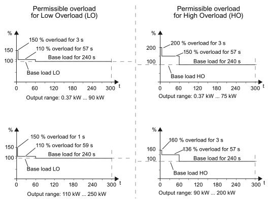
Figure 10-1 Duty cycles, "High Overload" and "Low Overload"
