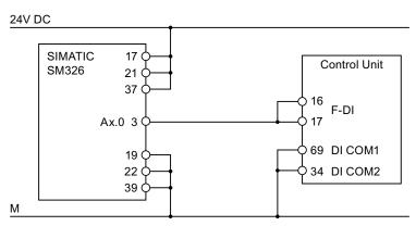
Figure 7-23 Connecting an F digital output module, e.g. SIMATIC F digital output module
