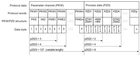
Figure 6-13 USS user data structure
