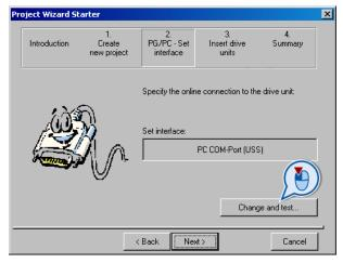
• Click "Change and test..." to set up the PG/PC interface.
