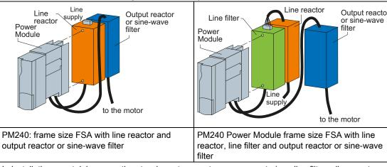
In installations containing more than two base-type system components (e.g. line filter + line reactor + output reactor), the components must be installed to the side of the Power Module whereby the line reactor and line filter are installed under the Power Module and the output reactor to the side.
