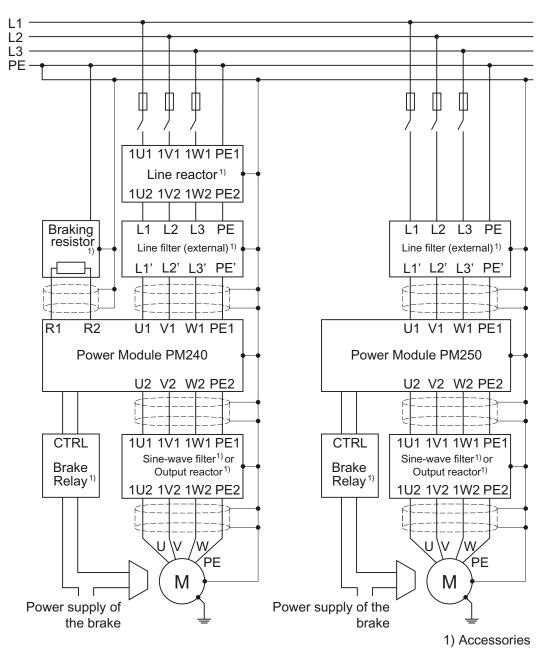
Figure 3-8 Connections for PM240 and PM250 Power Modules
