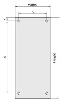
Figure 3-7 Dimensions and drilling pattern PM260
