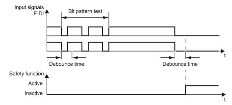
Figure 7-26 Filter for suppressing temporary signal changes
