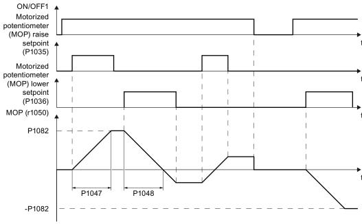
Figure 7-3 Function chart of motorized potentiometer
