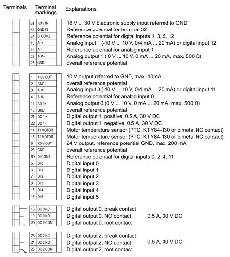
Figure 3-13 Terminal strip on CU240E-2, CU240E-2 F, CU240E-2 DP and CU240E-2 DP-F
