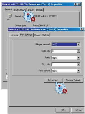
If the USB-COM emulation is assigned to an address higher than COM7, open the properties window by double-clicking on the interface. There you will find the "Advanced" button under the "Port settings" tab.
