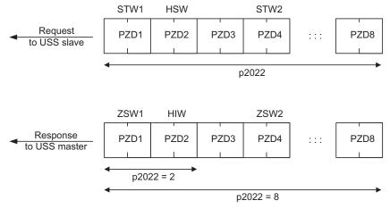
Figure 6-16 Process data channel
