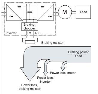
The inverter converts the regenerative power into heat using a braking resistor
