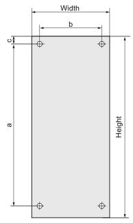
Figure 3-4 Dimensions and drilling patterns, PM250
