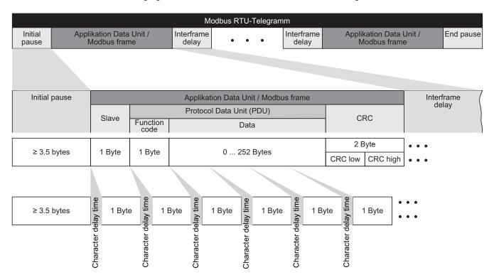
Figure 6-19 Modbus with delay times
