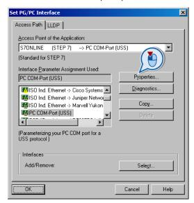
• If "PC COM-Port (USS)" is not available, click on "Select ..." to install the "PC COM-Port (USS)" interface as shown in the "Install/Remove Interfaces" dialog box.
