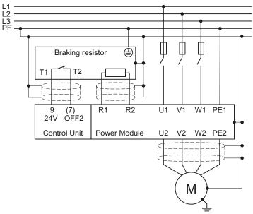
Figure 7-11 Braking resistor connection
