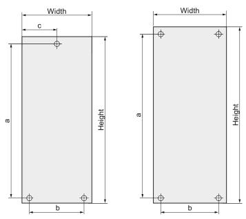
Figure 3-5 Dimensions and drilling patterns, PM250-2, IP20
