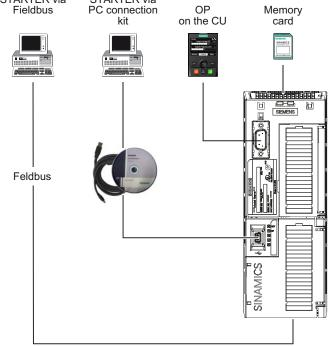
Figure 4-2 Inverter's parameterization interfaces
