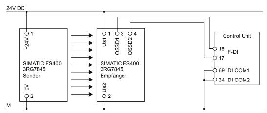
Figure 7-21 Connecting an electronic sensor, e.g. SIMATIC FS-400 light curtain
