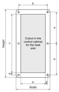
Figure 3-3 Dimensions and drilling pattern, PM240-2 PT
