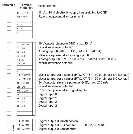
Figure 3-12 Terminal strip on CU240B-2 and CU240B-2 DP
