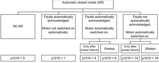
Figure 7-16 Selecting the automatic restart mode
