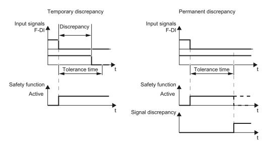
Figure 7-24 Filter for suppressing discrepancy monitoring
