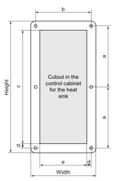
Figure 3-6 Dimensions and drilling pattern, M250-2, PT
