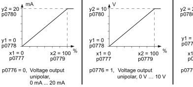
Figure 5-2 Examples for scaling characteristics
