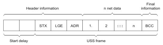
Figure 6-12 Structure of a USS telegram
