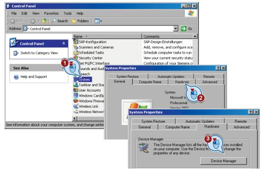
If the assignment lies in the range COM1 ... COM7, then you do not have to make any changes and you can close the control panel again. However, you should note the number of the COM interface as you will require it in a later installation step.
