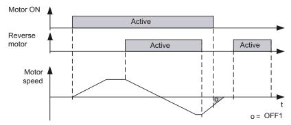
Figure 7-2 Motor control using digital inputs
