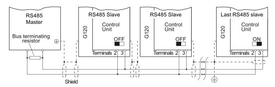
Figure 6-11 Communication network via RS485
