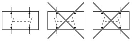
Figure 7-19 Sensors that can be connected to the fail-safe inputs
