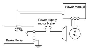
Figure 7-12 Connecting the motor holding brake
