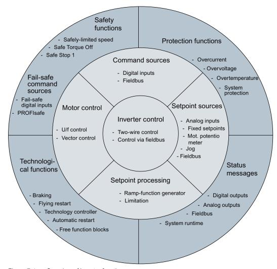
Figure 7-1 Overview of inverter functions
