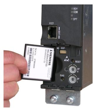
Figure 3-13 Slot for memory card
