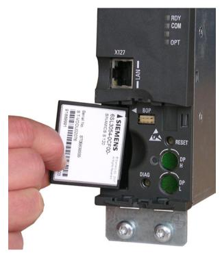
Figure 3-7 Slot for memory card
