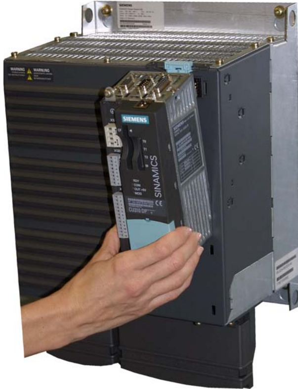
Figure 9-1 Mounting the CU310 onto the Power Module 340 (frame size D)
