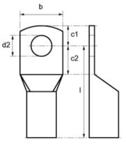
Figure A-1 Dimensions of the cable lugs
