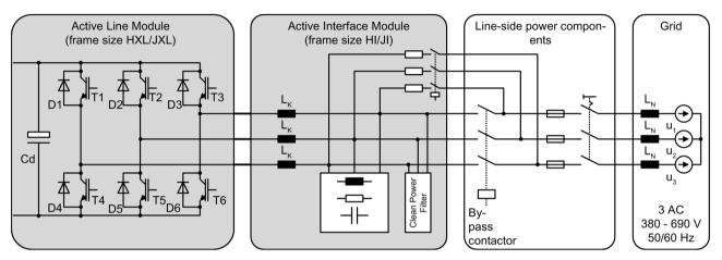
Figure 8-10 Overview of Active Infeeds, frame sizes HI/HXL and JI/JXL
