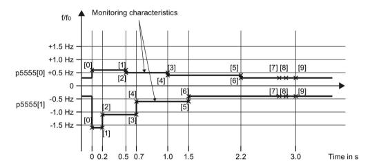
Figure 7-9 Example for frequency-time monitoring
