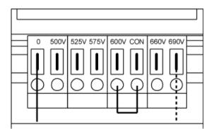
Figure 8-8 Setting terminals for the fan transformers (3 AC 380 to 480 V / 3 AC 500 to 690 V)
