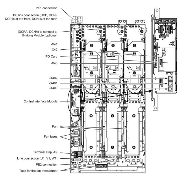
Figure 8-4 Active Line Module, frame size JX
