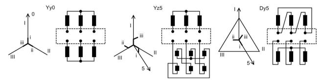
Figure 7-6 Connections and vector groups of three-phase transformers
