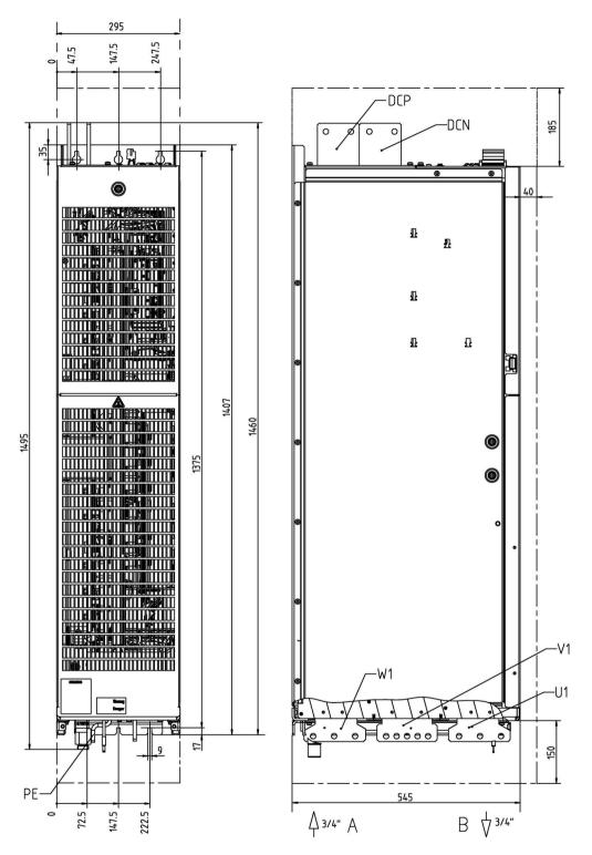
Figure 8-16 Dimension drawing Active Line Module, frame size JXL, article number 6SL3335-7TG41-6AA4. Front view, side view
