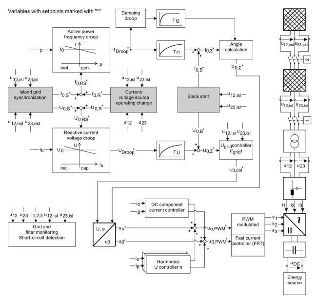
the generator inductances in the island grid. The downstream voltage controller ensures a steady-state accuracy of the voltage amplitude at the connection terminals, and therefore compensates the impedance of the inverter generating system.
