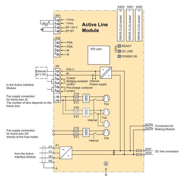
Figure 8-5 Active Line Module connection diagram
