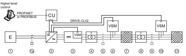
Figure 7-7 Configuration for the infeed in an island grid with coupling to the power grid – example, chassis format devices
