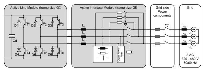
Figure 8-1 Overview of Active Infeeds, frame sizes GI/GX
