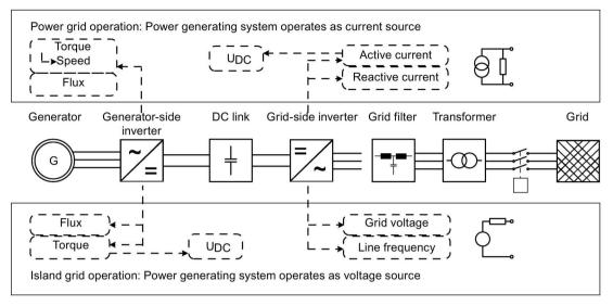
Figure 6-2 Basic control concept
