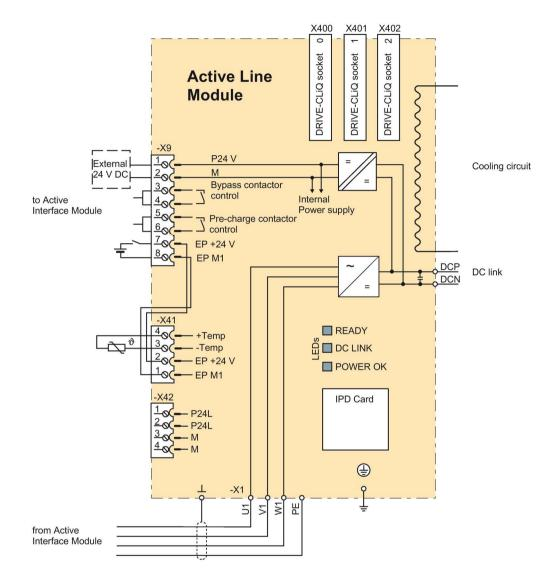
Figure 8-13 Example connection of Active Line Module
