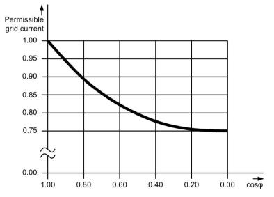
Figure 7-10 Derating characteristic for cos pot equal to one
