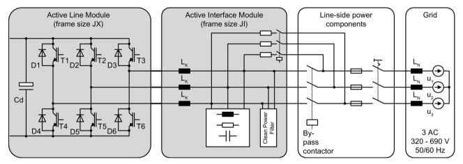
Figure 8-2 Overview of Active Infeeds, frame size JI/JX
