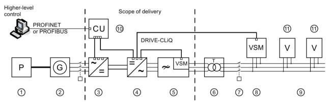
Figure 7-1 Infeed to a island grid via a generator
