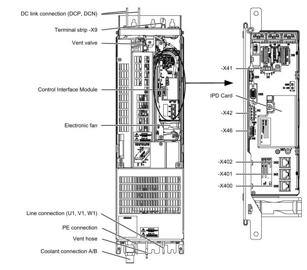
Figure 8-11 Active Line Module, frame size HXL
