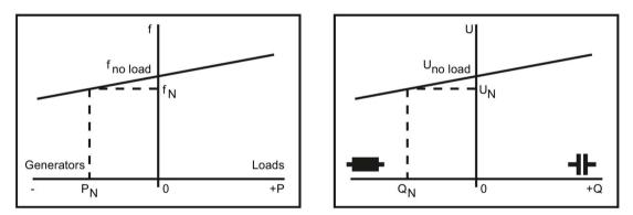
Figure 6-4 Active power droop characteristic and reactive power droop characteristic for frequency and voltage
