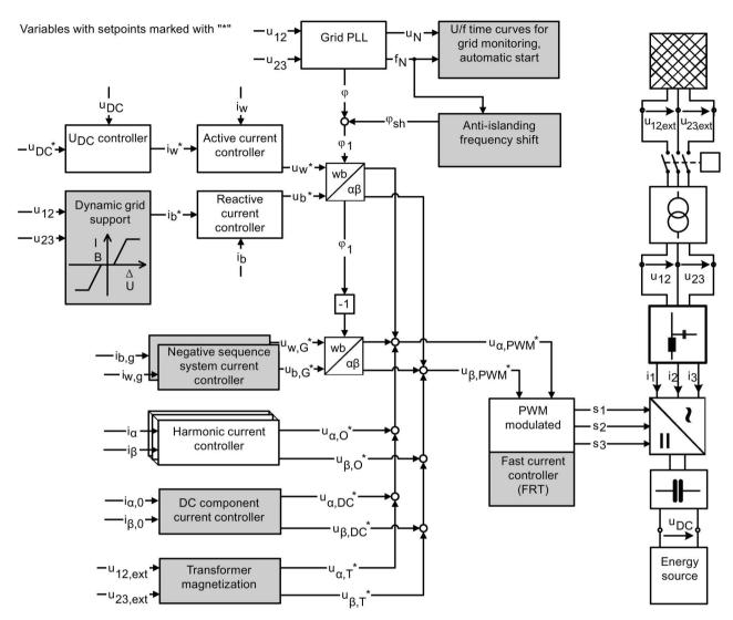
Figure 6-1 Additional modules for current-controlled operation
